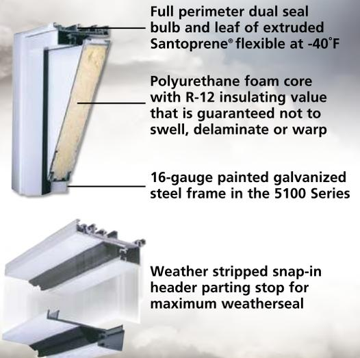
Full perimeter dual seal bulb and leaf of extruded Santoprene® flexible at -40°F
