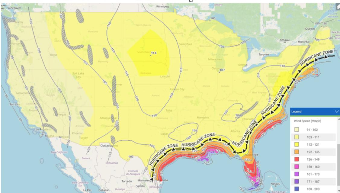
Figure 1: Hurricane Wind Load Map (image provided by ASCE 7 Online HAZARD TOOL: ASCE/SEI 7-16)
