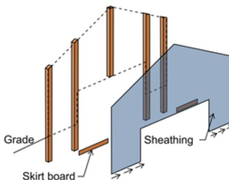
Figure 6: Multiple elements transfer lateral loads
