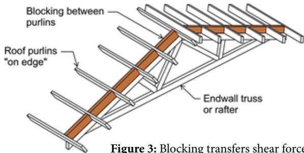
Figure 3: Blocking transfers shear forces.
