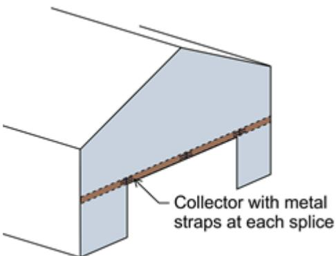
Figure 5: Collector members within shear walls
