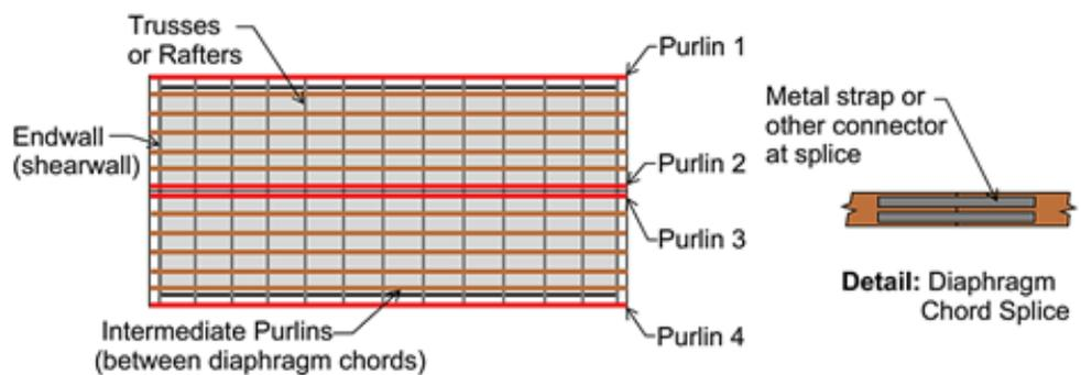
Figure 2: Roof diaphragm with some purlins as chords
