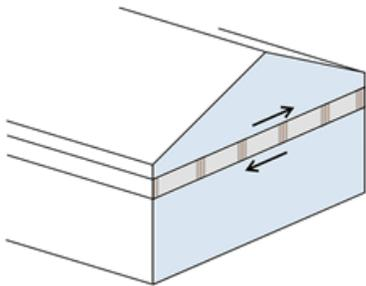
Figure 4: Shear Transfer complication at translucent panels
