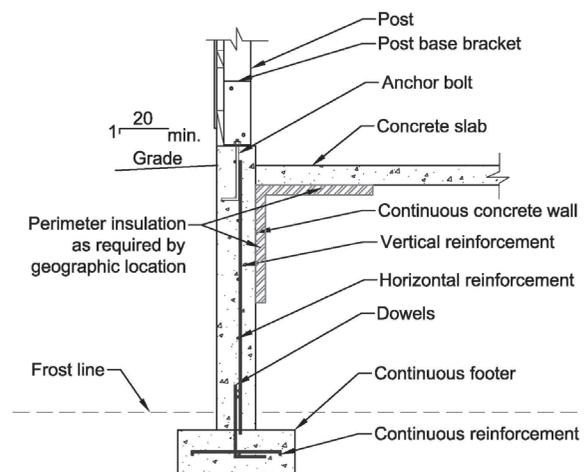
**Figure 3.** A continuous concrete wall foundation with a concrete floor. Posts are attached to the foundation with post base brackets.
