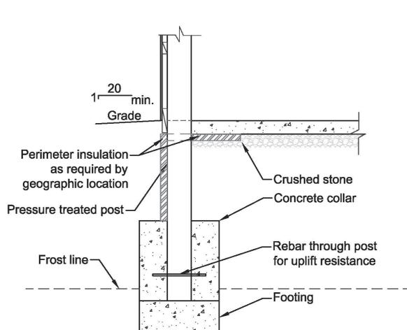
**Figure 2.** A constrained shallow-post foundation with a concrete collar and a concrete floor
