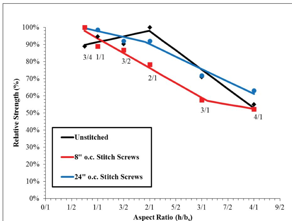
**Figure 7.** Relative design unit shear strength versus aspect ratio curve
