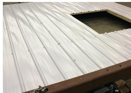
Figure 5. Buckling pattern for a shear wall with a 4' x 4' window. Note that the bottom fastening of the wall is obscured by the steel beam used to restrain out-of-plane movement during testing.
