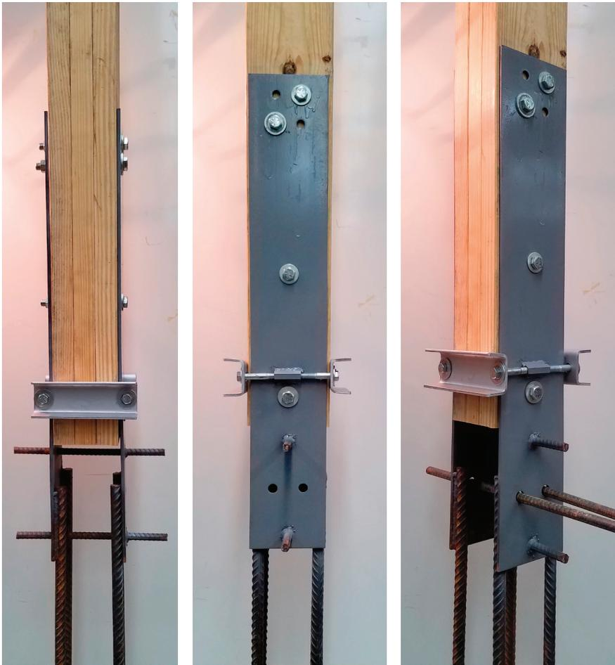
**FIGURE 10.** Front, side and angle views of a 2014 UW-Madison wood post-to-concrete connection design
