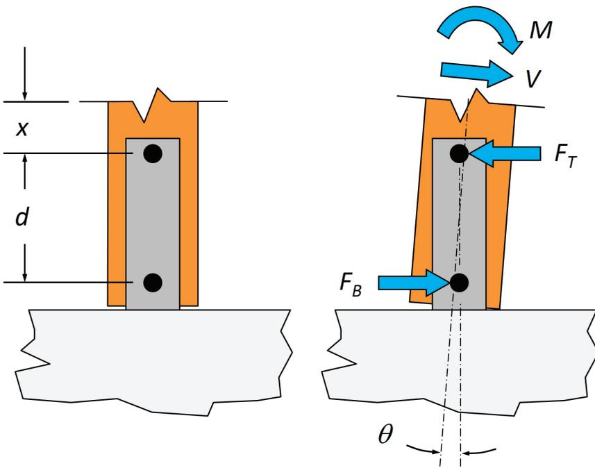
**FIGURE 7.** Forces applied to the wood post-to-concrete connection
