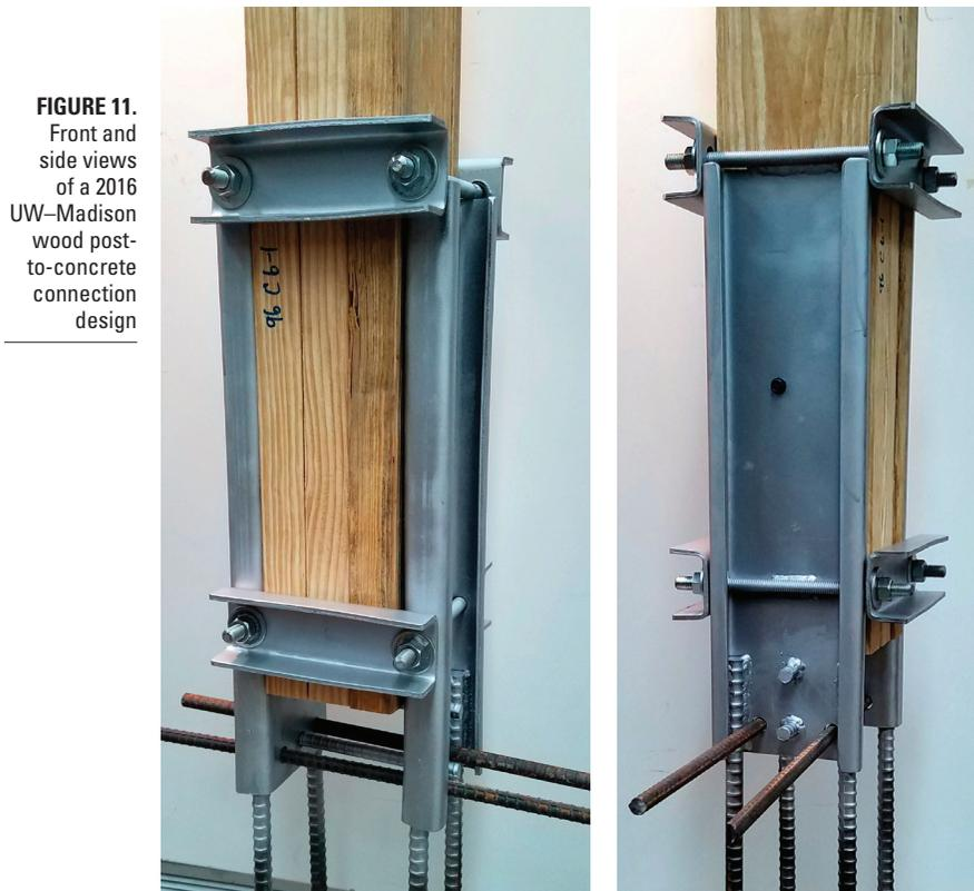
**FIGURE 11.** Front and side views of a 2016 UW-Madison wood post-to-concrete connection design
