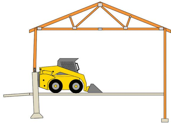
**FIGURE 5.** Connections must be designed to resist forces from equipment impact.
