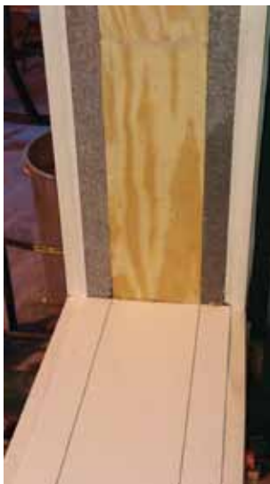
FIGURE 5. Installation of (a) specimen frame insulation around support beam, and (b) protective FRP skin
