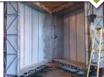
FIGURE 4. Climate (blue), specimen (black) and guard (red) trusses lined with steel panels
