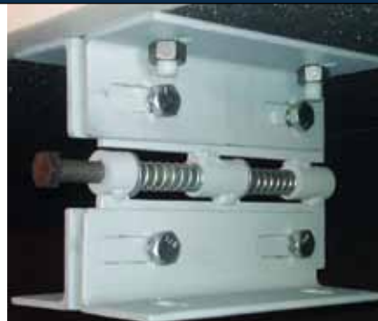
FIGURE 3. (a) Meter chamber and (b) meter chamber spring support
