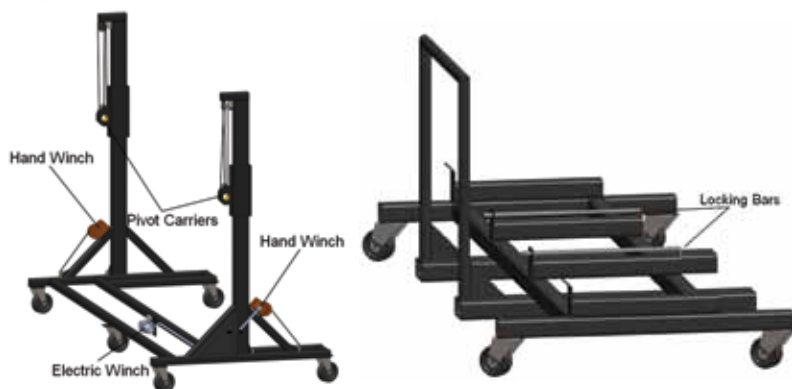
FIGURE 6. (a) Mobile base and (b) storage and transport cart designs
