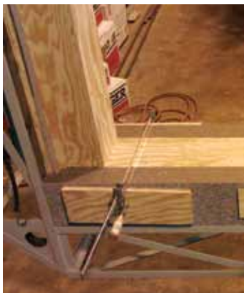
FIGURE 5. Installation of (a) specimen frame insulation around support beam, and (b) protective FRP skin
