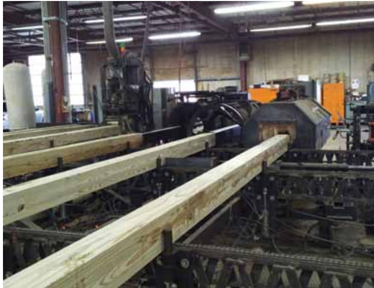
FIGURE 3. Automated application of an impermeable bitumen with ethylene propylene diene monomer encapsulation system. (Source: Barry Hoffman)
