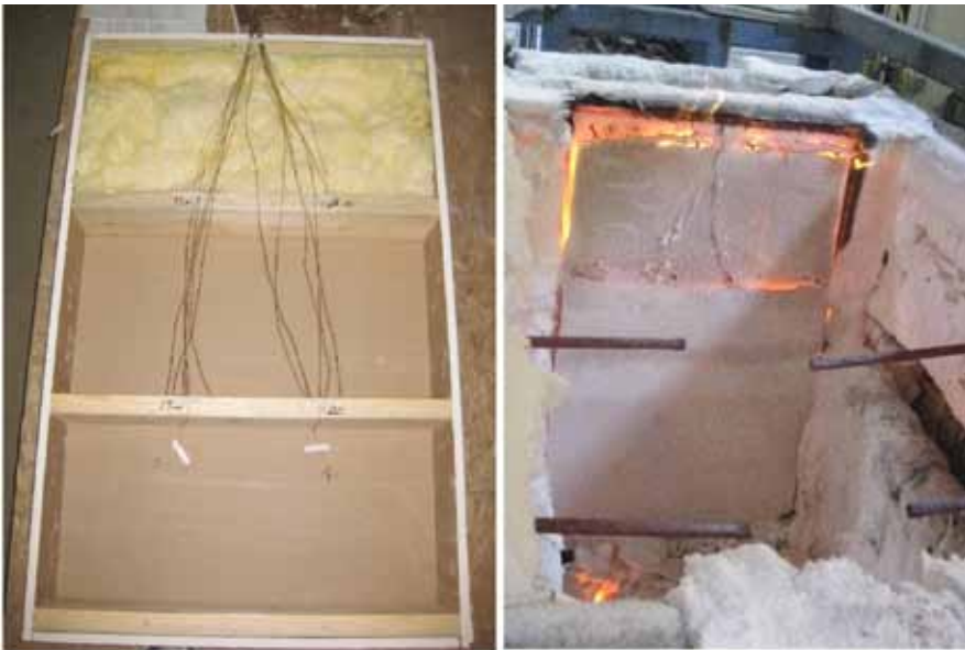
Figure 5. Left: upper fiberglass-insulated cavity (30 inches wide x 16 inches high) prior to sheathing; right: tested sample showing early sheathing failure in that upper cavity.
