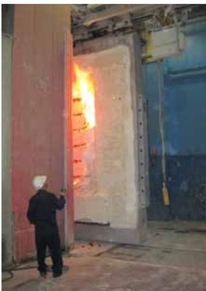
Figure 1. Full-scale testing of a post-frame fire-wall assembly
