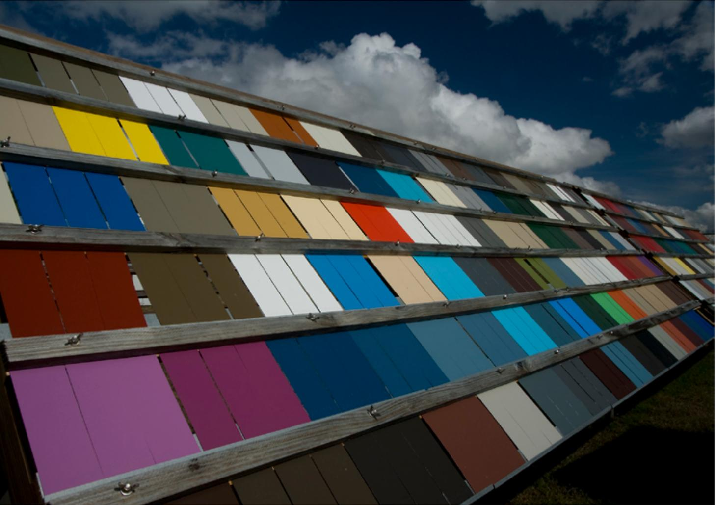
Weather testing is a critical variable to engineers when they are formulating new materials or improving upon old formulas.
