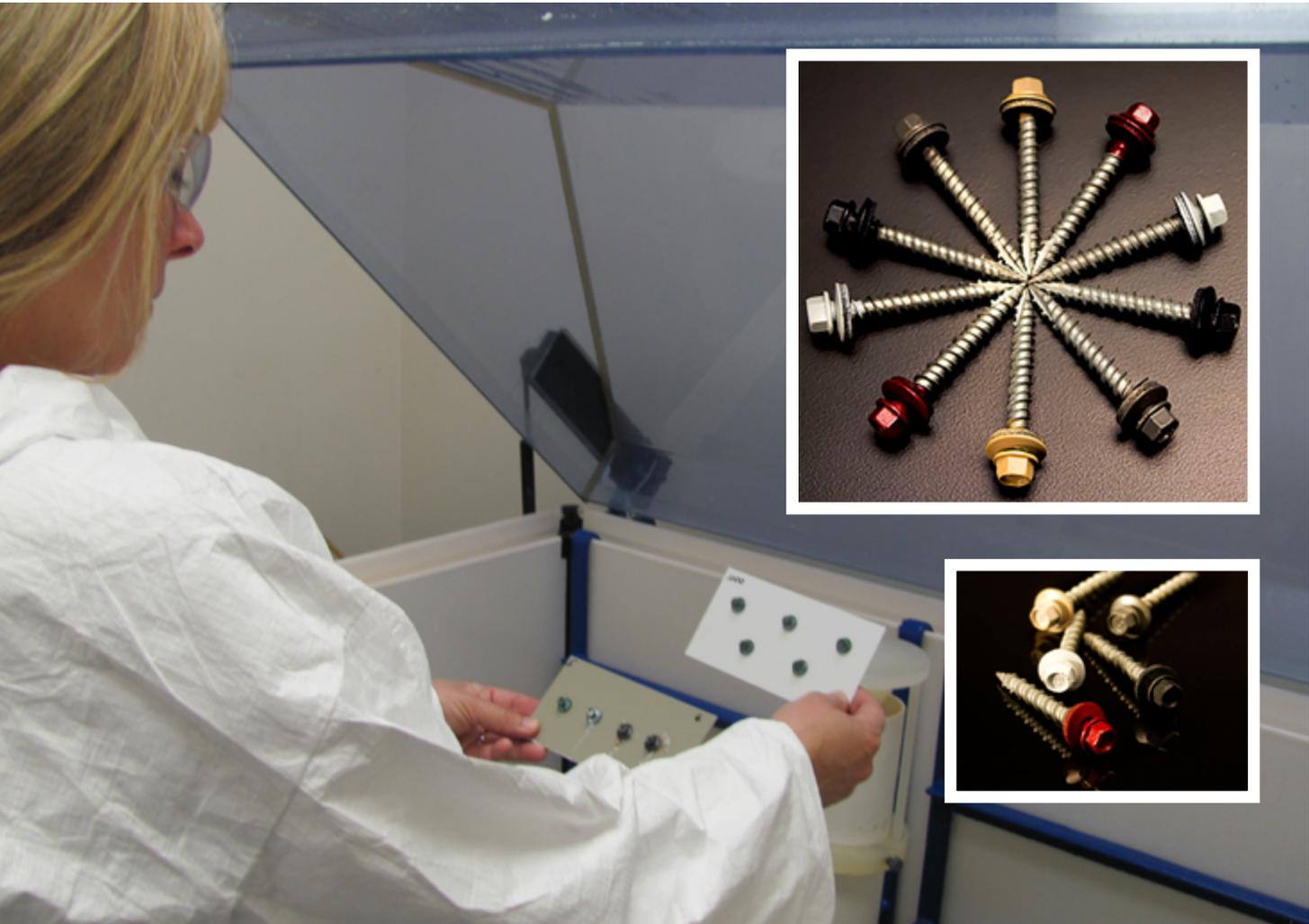
In a controlled environment within a laboratory, fasteners are subjected to a steady spray of salt water
