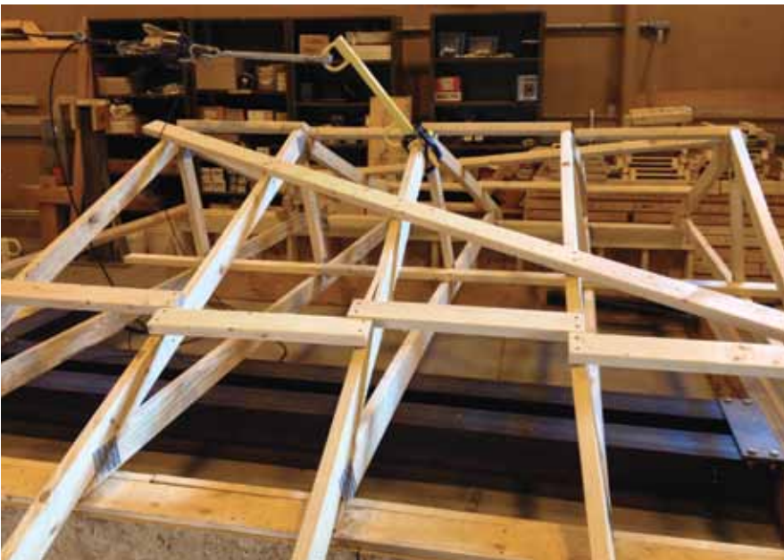
Figure 4. Loading of five-truss system with over-the-top bracing and splitting of truss top chord at center
