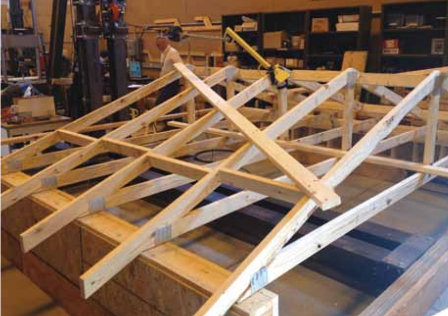
Figure 3. Five-truss system with blocking showing bracing pullout near PFAS
