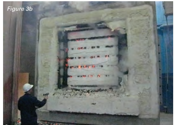
Figure 3. Full-scale post-frame fire-wall testing.
