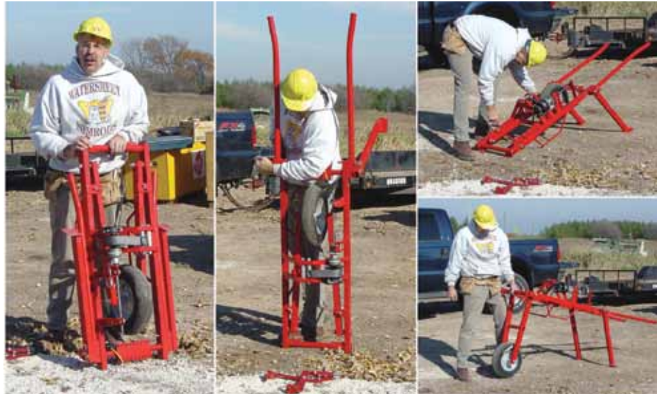
To unfold Big Dave's Cookie Cart (1) stand the cart on its front (left), (2) unfold the legs and handles and pin them in place (center), (3) lower the cart so it is resting on its legs (upper right), and (4) swing and lock the wheel frame into place (lower right).
