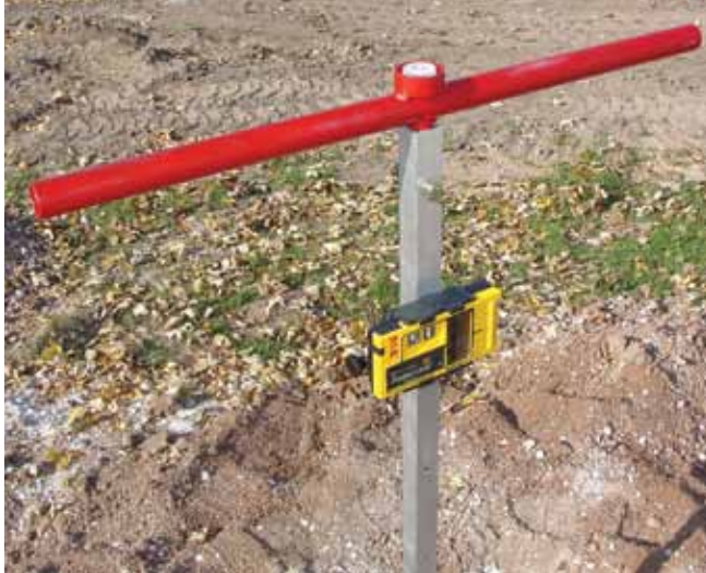
Figure 8. T-bar handle on the Badger Hole Leveler contains a bull's-eye level. Square outer tubing of the telescoping shaft facilitates attachment of a laser level receiver.
