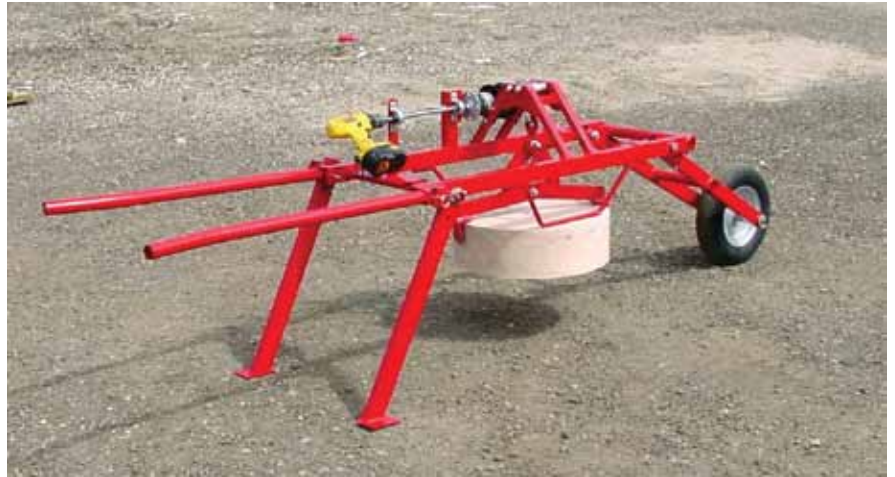
Figure 10. The latest version of the footing transport and placement cart during a recent test. Drawn to the underside of the cart is a 6-inch thick by 20-inch diameter precast concrete footing weighing approximately 165 lbm.
