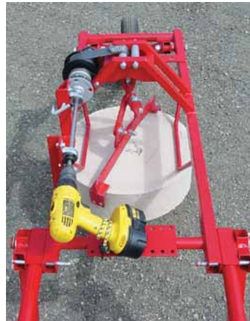
Figure 11. Top view of the footing transport and placement cart.
