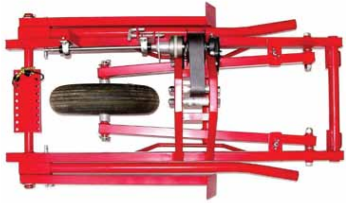
Figure 13. Side and top views of the footing transport and placement cart after it has been folded for storage. Note from the top view that when folded for storage, the cart can still be moved about like a wheelbarrow.
