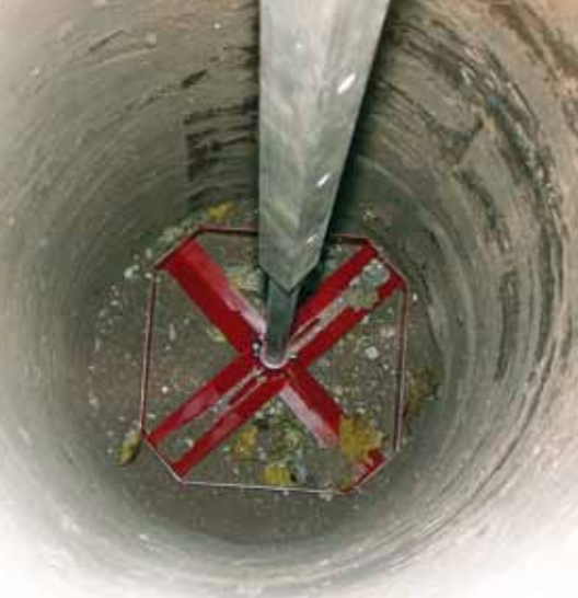
Figure 7. The Badger Hole Leveler in use. Note telescoping shaft consists of round aluminum stock that slides inside a square aluminum tube.
