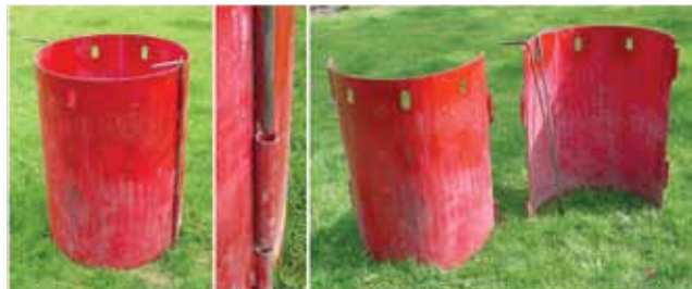
Figure 1. The Wisconsin Hole Shield (left) is separated into two halves (right) by simply withdrawing two L-shaped pins (center).
