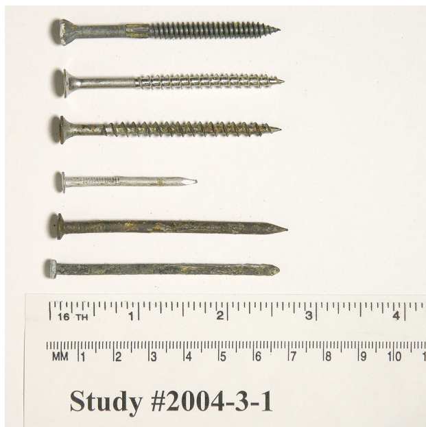
Nails and screws in contact with ACQ-D treated wood for six months. The treated wood was put in a conditioning room with 100 percent relative humidity at 80 degrees Fahrenheit. The fasteners are (top to bottom): a proprietary coated fastener, stainless steel, electroplated galvanized, aluminum, plain carbon steel, and hot dipped galvanized.
