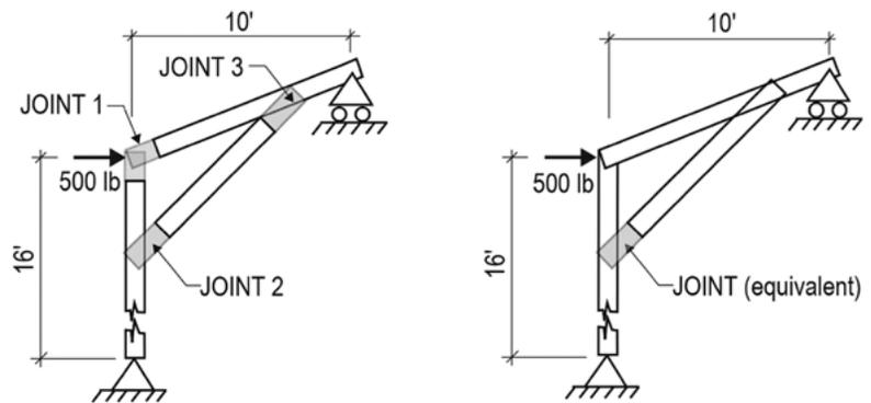
**Figure 2:** Knee brace with slip at all joints (left) and with an equivalent slip at one joint (right)
