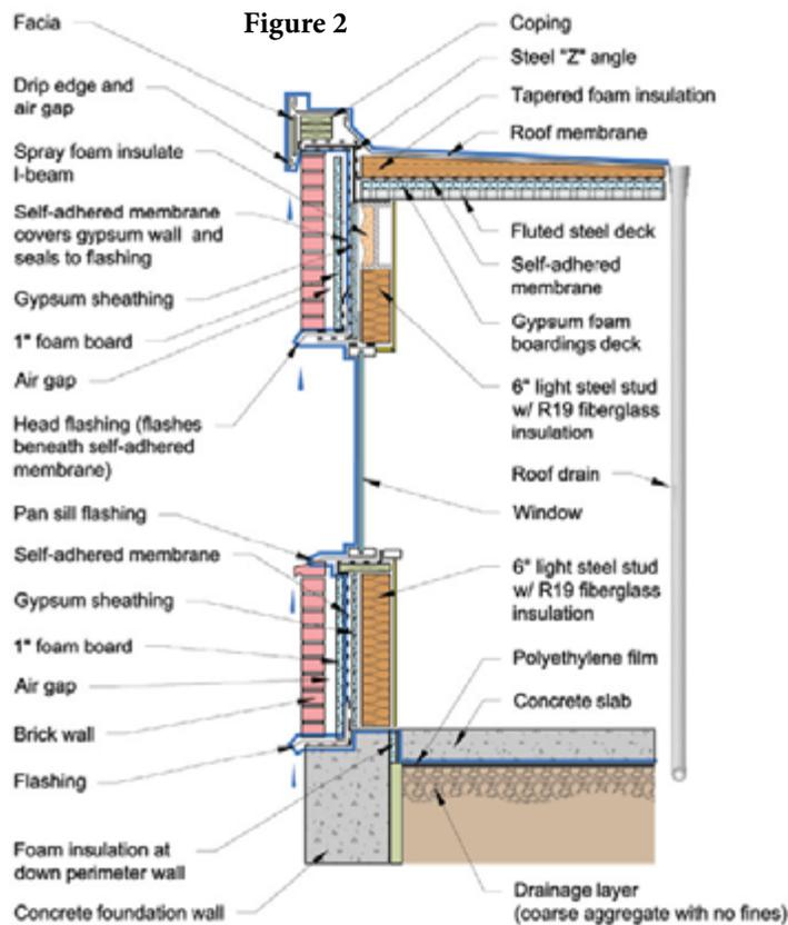
**Figure 2:** A "Pen Test" can help determine if the chosen design will protect the building from rainwater moisture penetration. This example
