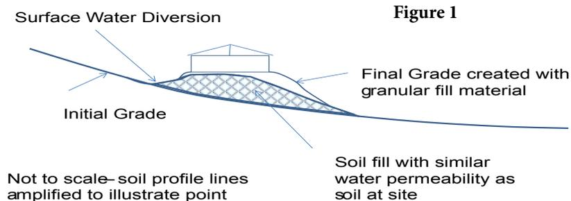
**Figure 1.** This illustrates how low permeability fill should be placed to ensure that infiltrated surface water does not collect under the new building base.
