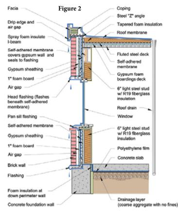
**Figure 2:** A "Pen Test" can help determine if the chosen design will protect the building from rainwater moisture penetration. This example
