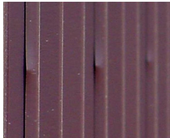
Figure 3 - Example of edge kinking.
